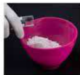
Step 02 Pour in the powder measure (10 g) and then add the water (19 mL)
